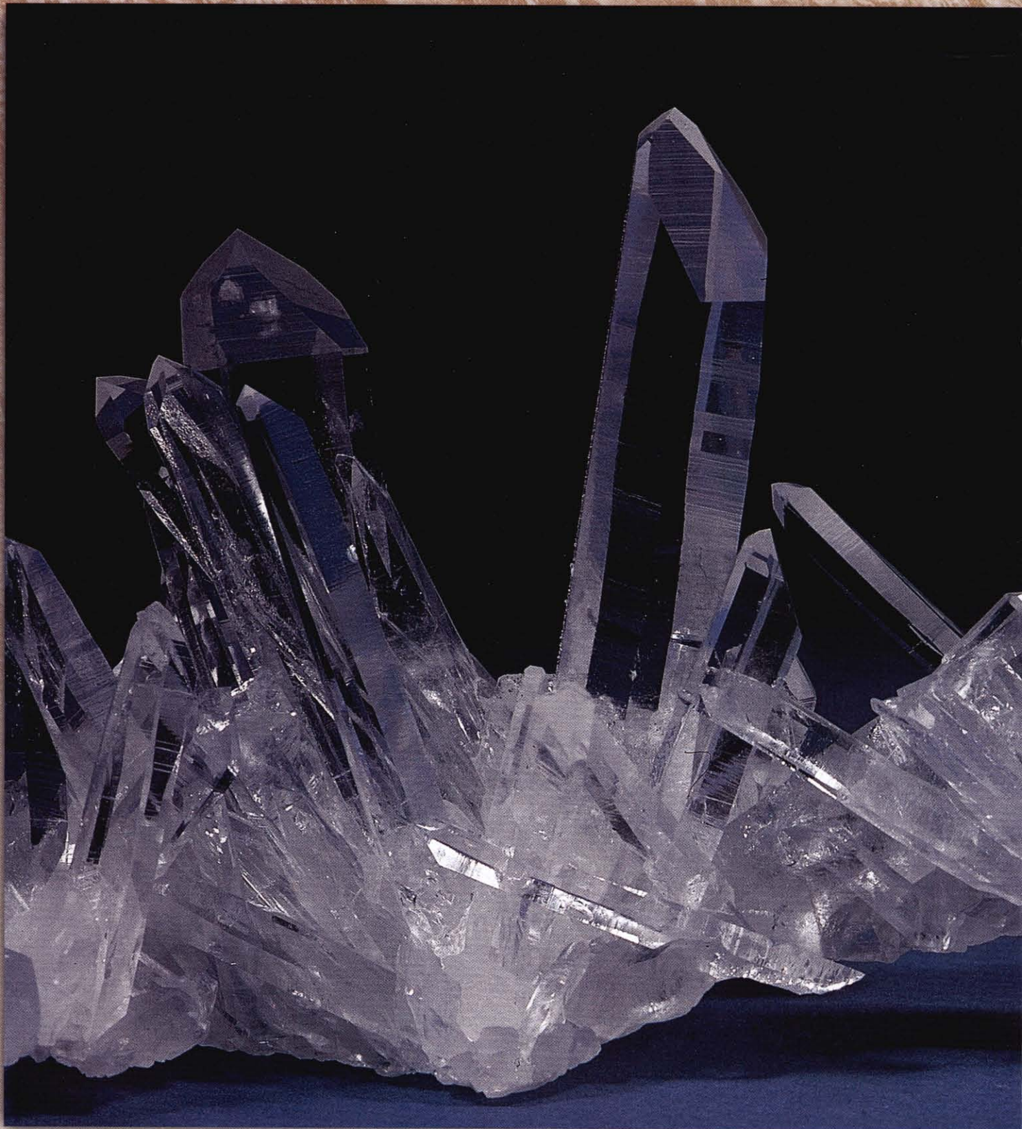
Crystals of amethyst, a variety of quartz. The planar surfaces are crystal faces, whose geometries are determined by the underlying arrangement of the atoms that make up the crystals. [Breck P. Kent.]
