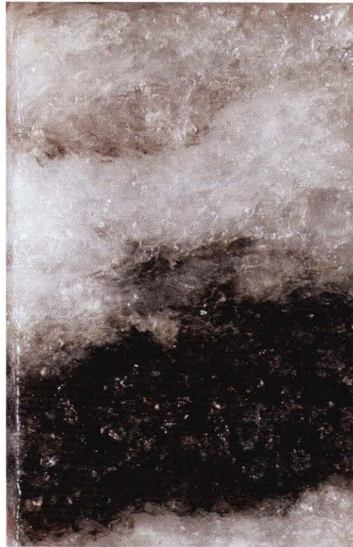
Figure 3.10 A halite deposit from the Sultanate of Oman. This deposit, which is more than 500 million years old, is preserved in a drill core from the deep subsurface. The black band is concentrated organic matter derived from microorganisms that lived in extreme hypersaline environments that formed when the ancient ocean dried up. [John Grotzinger.]
