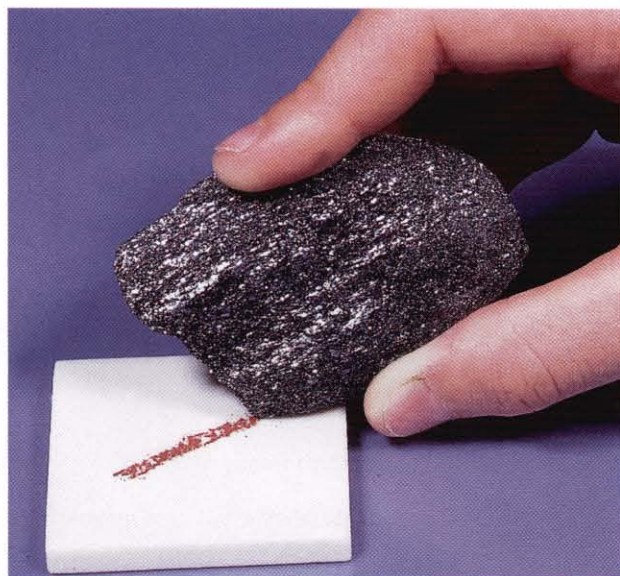
Figure 3.20 Hematite may be black, red, or brown, but it always leaves a reddish brown streak when scratched along a ceramic plate. [Breck P. Kent.]
