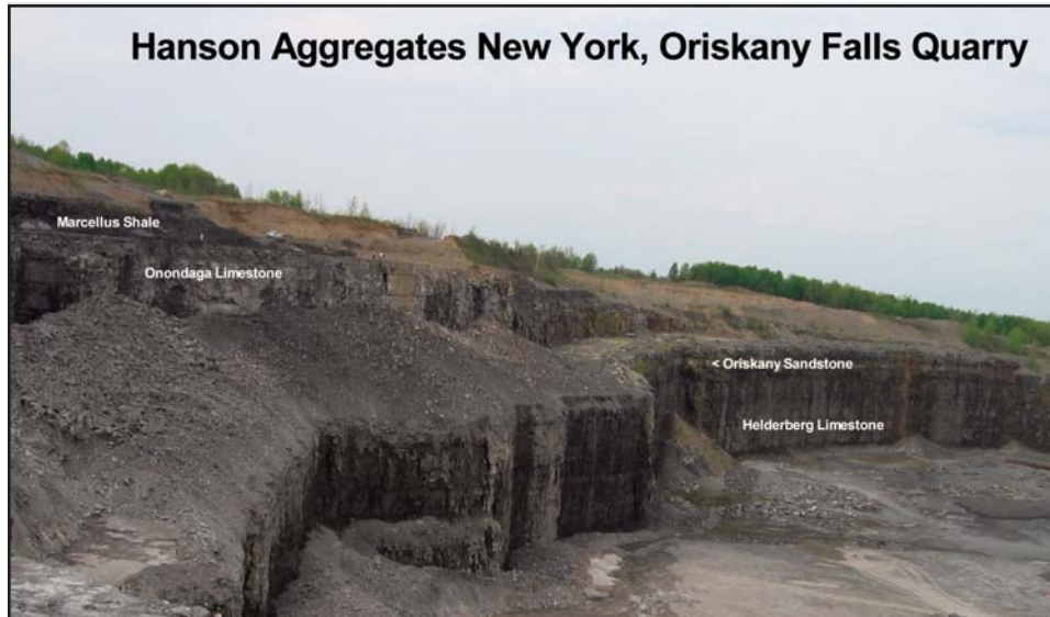
Figure 5. Hanson quarry at Oriskany Falls, New York. Marcellus Shale is at the top left, near the white truck. The base of the Marcellus is the top of the Onondaga Limestone at the upper bench. The Oriskany Sandstone is identified in the quarry wall a short distance below the second bench as a yellowish layer below a small slope break. The rock below the Oriskany is Helderberg Limestone, which is the main production from this quarry. Photograph by Daniel J. Soeder.
