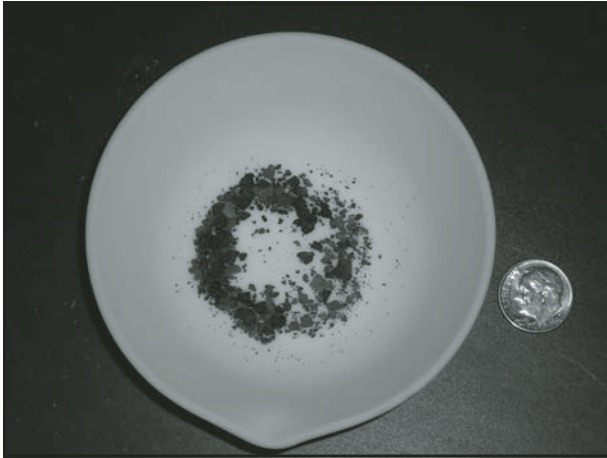
Figure 37. Washed and dried Marcellus Shale drill cuttings displayed in a laboratory dish. Coin shown for scale is 18 mm in diameter. Photograph is by Daniel J. Soeder.
