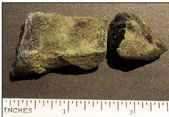
Figure 40. Weathered Marcellus Shale outcrop samples from Franklinton, Pennsylvania, coated with tiny crystals of yellow sulfur, presumably left behind from the oxidation and leaching of sulfide minerals such as pyrite. Photograph is by Daniel J. Soeder.
