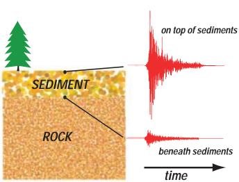
When waves of a small earthquake impinge on the boundary between hard rock and overlying sediments from below (lower seismogram), they become amplified as they travel through the sediments to the surface (upper seismogram). A seismogram records the wave motion over time. The amplifying effects of thick sediments above the New Madrid seismic zone results in motions at the surface that are many times larger than below. (Courtesy of C. Langston, The University of Memphis.)
