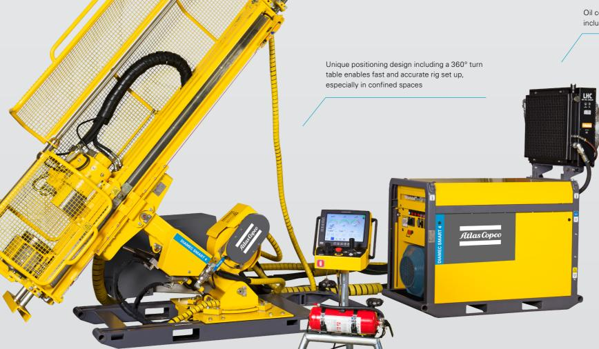
A-N rotation unit with sealed gear box, hollow spindle and hydraulic chuck. The chuck and rod holder are synchronized and the rotation unit and rod holder come with a hinge design
