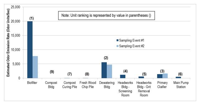
Figure 3: Estimated Odor Emission Rate and Unit Ranking For Potential Mitigation Efforts from Two Sampling Events. Note: The compost building is exhausted through the biofilter. Therefore, no direct emissions are expected.
