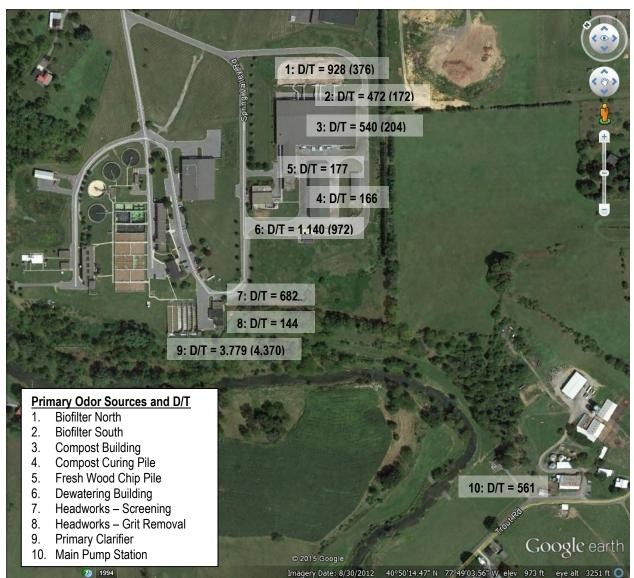
Figure 2: Detection Threshold for Primary Odor Sources from Sample Event #1 and (Sample Event #2)
