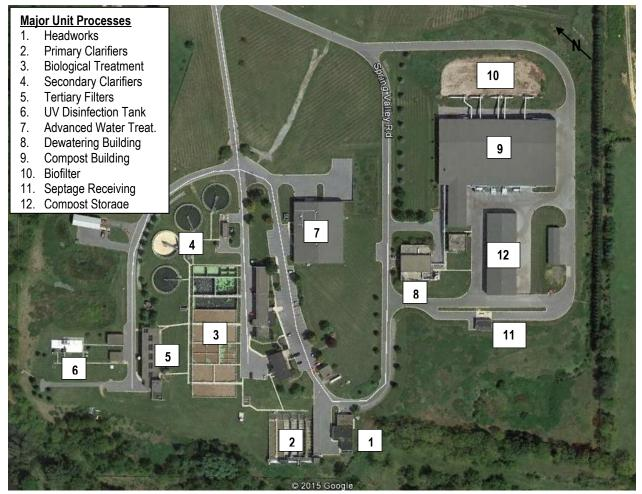
Figure 1: Aerial View of the SCPCF Illustrating the Facility Layout and Identification of Unit Processes (Image Source: Google Earth)
