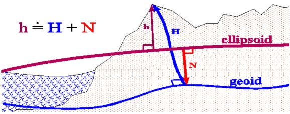
*Figure 2-1. Relationship between ellipsoidal (h), orthometric (H), and geoid (N) heights.*
