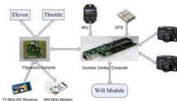
Fig. 8. AggieAir Airborne System Structure.
