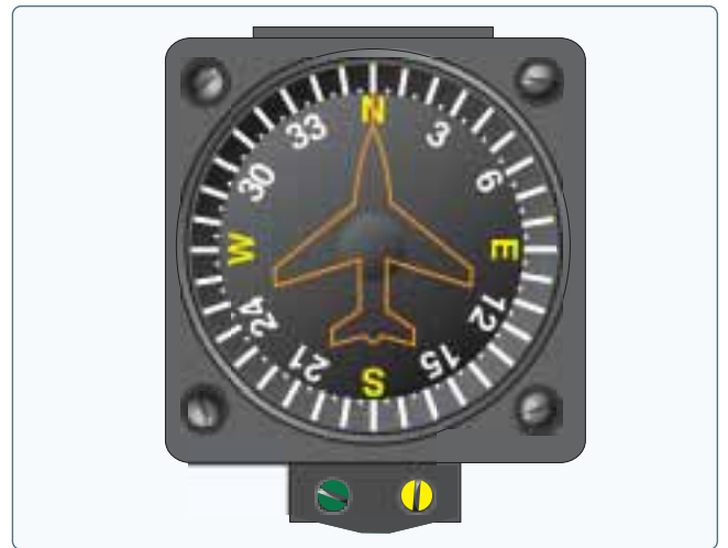
Figure 8-38. Vertical card magnetic compass.
