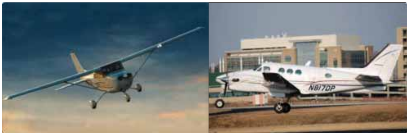
Figure 7-39. Fixed (left) and retractable (right) gear airplanes.
