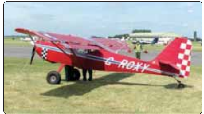
Figure 6-9. Flaperons on a Skystar Kitfox MK 7.
