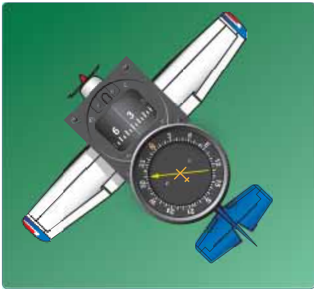
Figure 16-37. ADF with fixed azimuth and magnetic compass.
