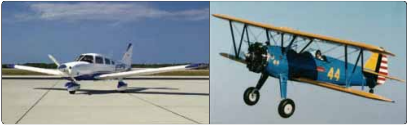
Figure 3-6. Monoplane (left) and biplane (right).
