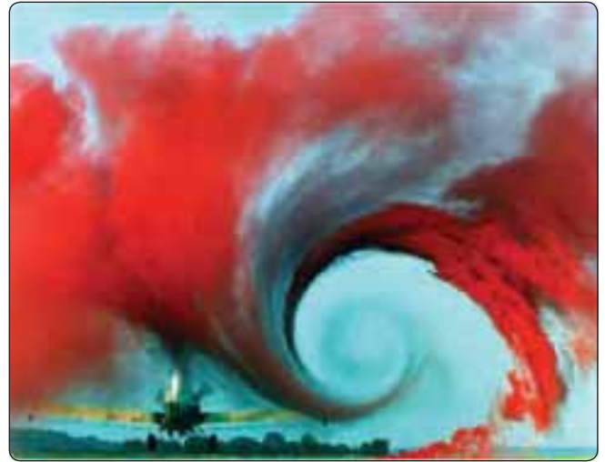
Figure 5-9. Wingtip vortex from a crop duster.
