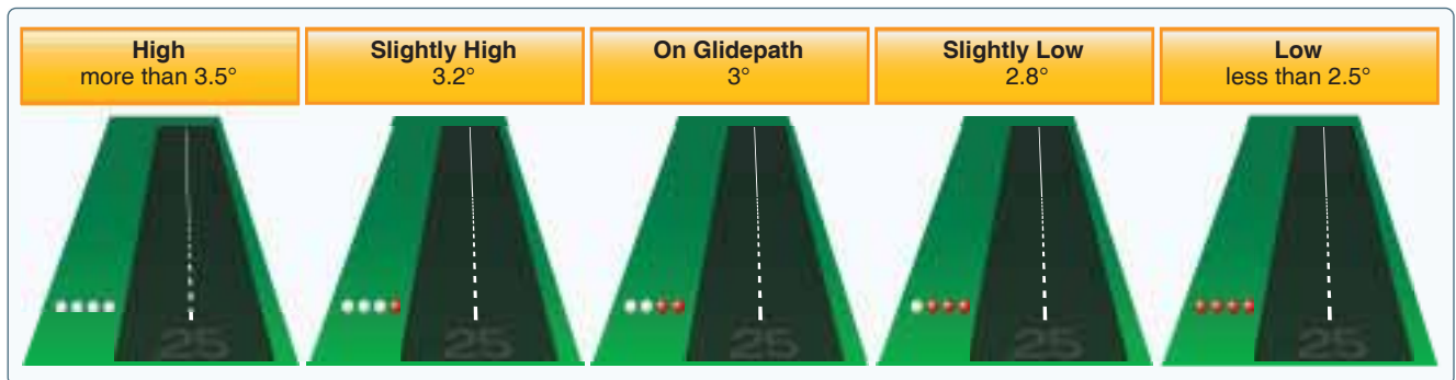
Figure 14-30. Precision approach path indicator for a typical 3° glide slope.
