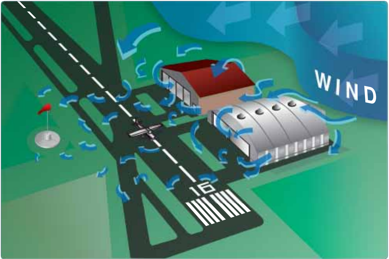
Figure 12-15. Turbulence caused by manmade obstructions.
