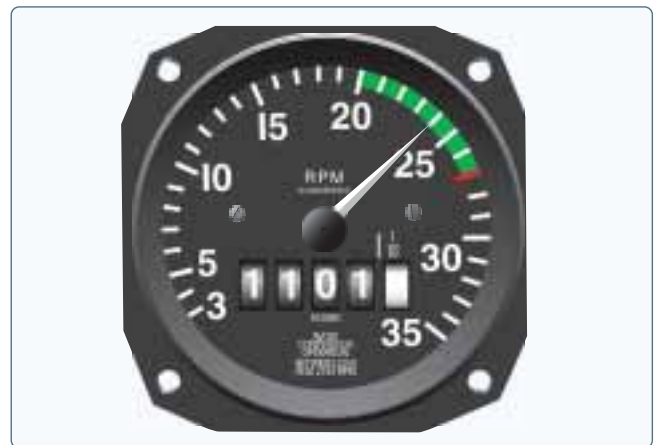
Figure 7-8. Engine rpm is indicated on the tachometer.
