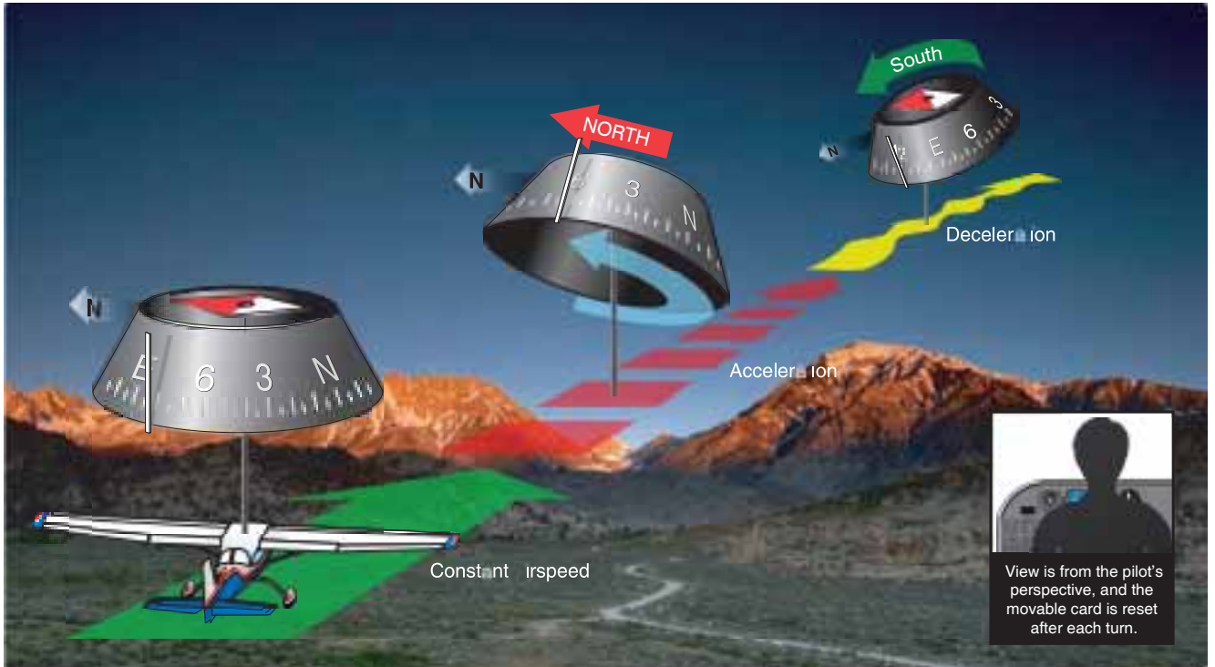
Figure 8-37. The effects of acceleration error.
