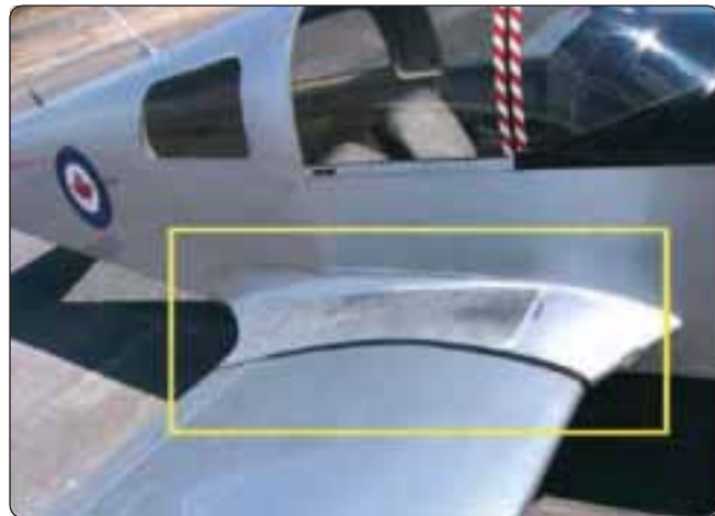
Figure 5-8. A wing root can cause interference drag.
