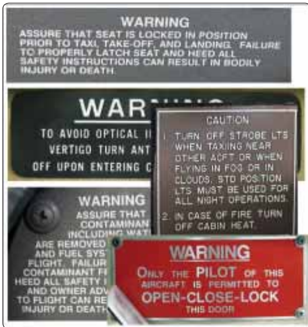
Figure 9-5. Placards are used to depict aircraft limitations.
