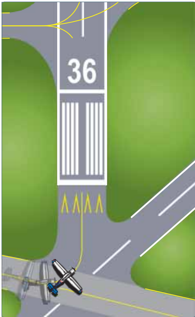
Figure 14-49. Confusing runway/runway intersection.
