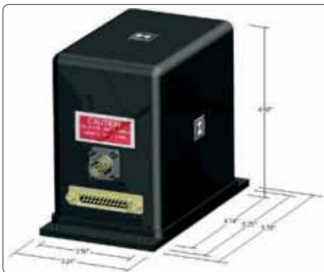
Figure 8-26. Attitude and heading reference system (AHRS).
