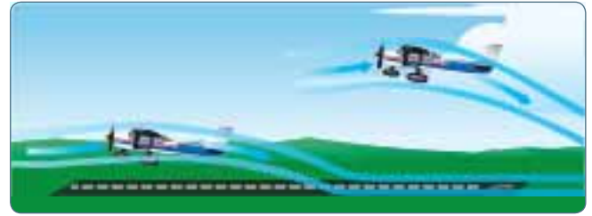
Figure 5-16. Ground effect changes airflow.
