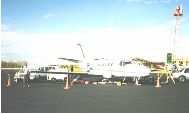
Figure 6. Window Ported NOAA Cessna Citation Undergoing Spatial Offset Measurements at Springfield, Ohio
