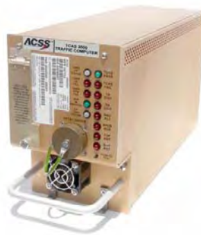
Figure D-15. The M 2 CAS Chassis Housing TCAS and Data Fusion Functions
