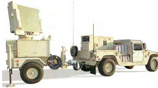
Figure 12. Transportable TRS Sentinel Radar
